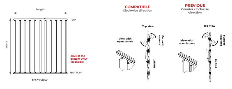
The above drawing should be interpreted as a front projection of the system. Mounting of the SUNBREAKER 210 system can be carried out in a niche or on a substructure. NO FACADE MOUNTING BRACKETS!!!
